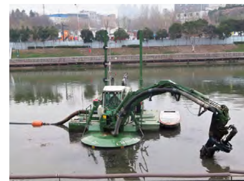
Watermaster is an environmental dredger it works extremely efficiently and accurately, being able to remove very precise layers of sediments while causing a minimal amount of turbidity.
